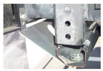
Driver Side View: Skid mounts to the outside lower bumper bolt on the top. The skid mounts to the outside hole on the stock under-rider bar as shown.
