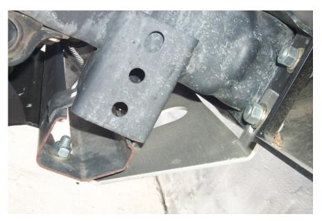
All 2012 and later model Jeep JK's will require minor trimming of the factory gusset found on the lower under-rider bar. Photos below show where to mark and trim for skidplate clearance.
